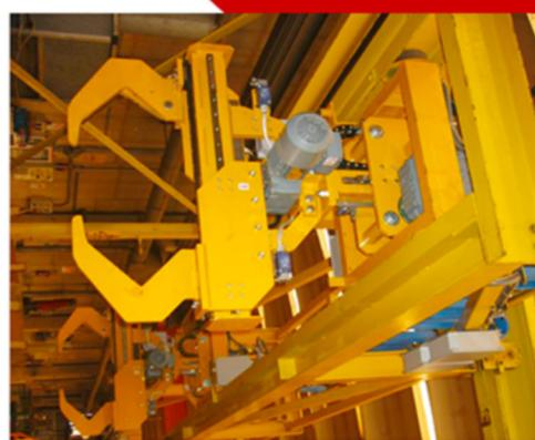
Multi-axis automatic overhead cranes able to move the materials during the working phases; it's an automatic bridge crane able to move heavy and continuous loads. The purpose is to automate processes, in a completely safe and reliable way, that would be difficult, dangerous and expensive to handle manually with traditional systems.
